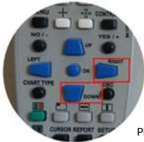
Pic.4. [RIGHT] and [DOWN] arrow button on remote control.
